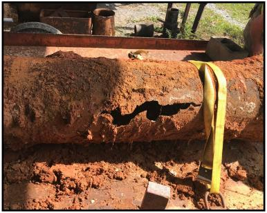
Failed Ductile Iron Pipe – 9 years old.
